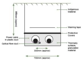
The cable ducts will be laid circa 300mm apart to achieve thermal independence, alongside fibre optic cables installed in a separate duct, within a bedding of thermally suitable compactable granulated material, such as cement-bound sand (CBS). The remainder of the trench will be reinstated within a bedding of indigenous sub-soil, overlain by topsoil.
