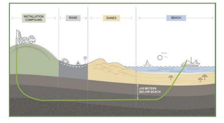
Figure 2-1 Illustration showing how HDD might work
